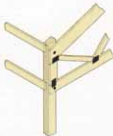
Deep Heel Trusses offer lower-profile roof pitches with unobstructed wall to ceiling corners
