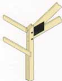
Deep Heel Trusses offer lower-profile roof pitches with unobstructed wall to ceiling corners
